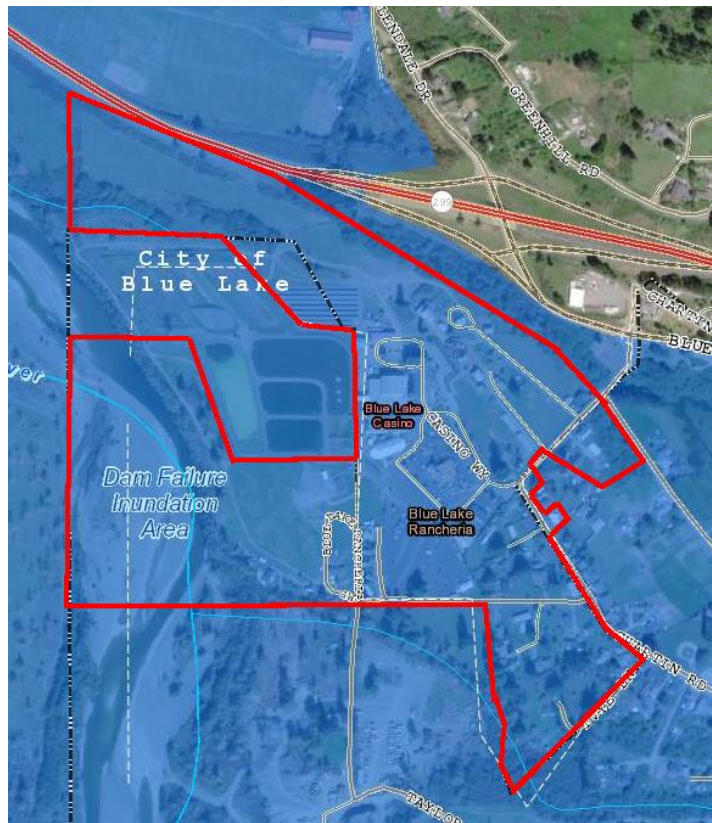
Figure 4.16 - R.W. Matthews Dam Failure Inundation Model
